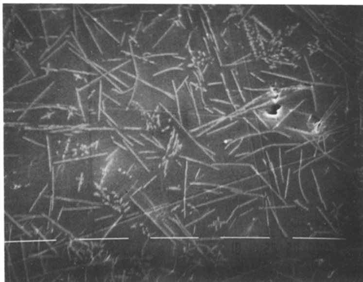
Figure 3 Rutile needles grown by crystallizing the glass for 0.5 h at 1000°C. White bar = 10 \mu\text{m} .
